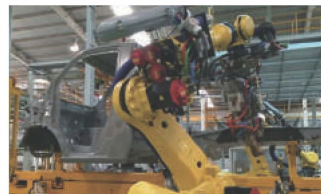
Pengelasan system robotic
